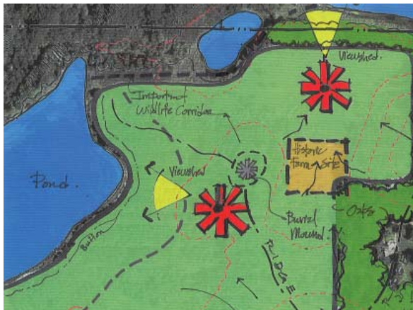
A site inventory and analysis highlights the opportunities and constraints of a property, such as drainage patterns, access, historic sites, viewsheds, wooded areas, wildlife corridors, and water resources.
