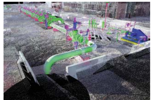
"Point cloud" of 3D data generated by the laser scanner
